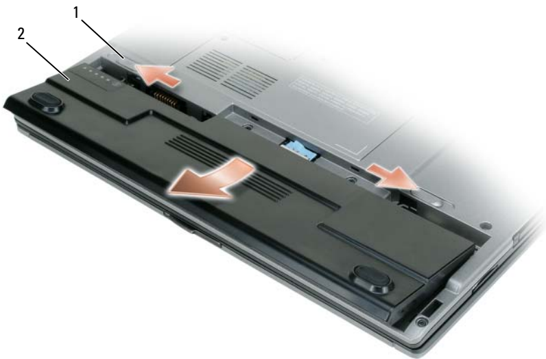
1 battery-bay release latch (2) battery
